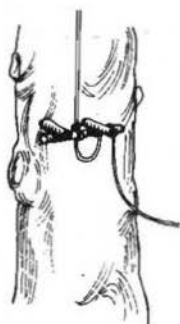
A trigger for a deadfall/snare combination.
